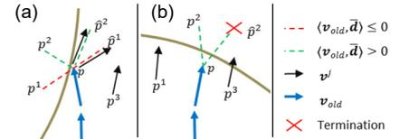
**Fig. 1:** Illustration of the voting process leading to a streamline reflection (a) and a termination after the next one or two steps (b).
